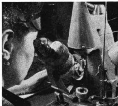
HOLES IN THE HEART OF A DIESEL are drilled by Marion Olszanecky at General Motors' Diesel Equipment Division. Drills used are nearly invisible to the naked eye.
