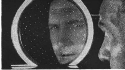
THROUGH THE LOOKING GLASS — a metal spinnerette used in the manufacture of synthetic yarns—come tiny beams of light. Holes, less than 1/1000-inch in diameter, are made by John Cupler's microscopic drills.
